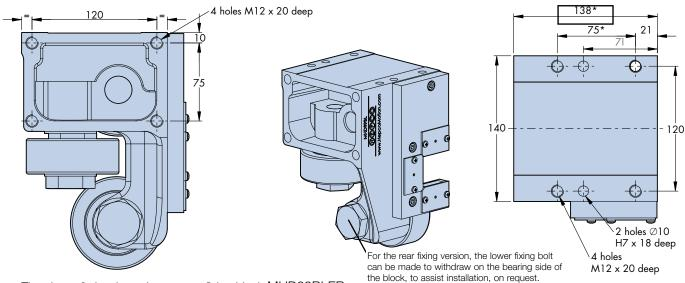
The above 3 drawings show a rear fixing block MHD89BLER
