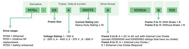
For configurations involving frame size 9 and above refer to the Unidrive M: High Power Modular AC Drives brochure
