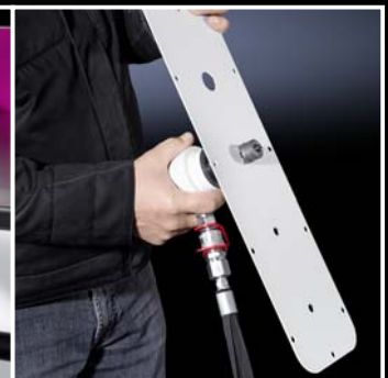
Making cut-outs in steel and stainless steel (accessories, hydraulic hose and cylinder, see page 645)
