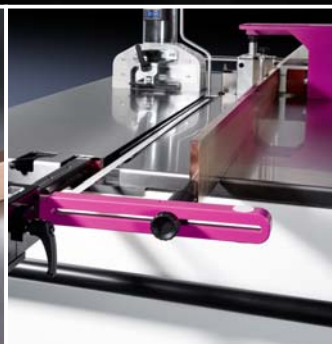
Punching busbars, pull-out measurement system
