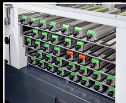
Stocking of up to 80 magazines for terminal blocks, miniature fuse-breakers etc.
